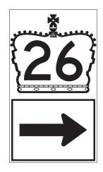
450 mm x 750 mm 600 mm x 1050 mm 900 mm x 1500 mm (b) M114 - Combination Marker -Provincial Crown with Cardinal Direction and Arrow
