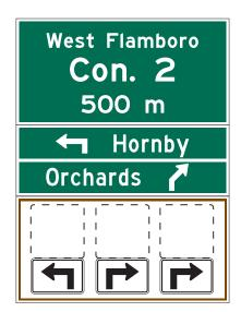
(d) Turn-Off Guide and Information Sign Assembly with Roadway Identification and Services Marker Board
