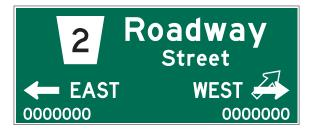
750 mm x variable width (Single Lane STOP-controlled exit)
