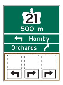
(b) Turn-Off Guide and Information Sign Assembly with Roadway Identification, Destination and Services Marker Board
