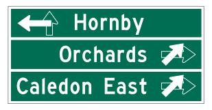
900 mm x variable width (Single Lane STOP-controlled exit)
